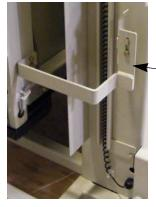
Switch positioning bar in storage position
